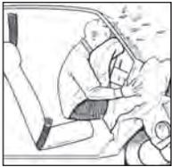
Air bags are more effective when you're buckled up and can be dangerous if you're not. You should be seated at least 10" away from the air bag as measured from the center of the steering wheel to your breastbone.
